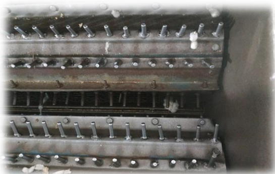
b - View of the cotton ginning zone using ten mm diameter pegs drums.
