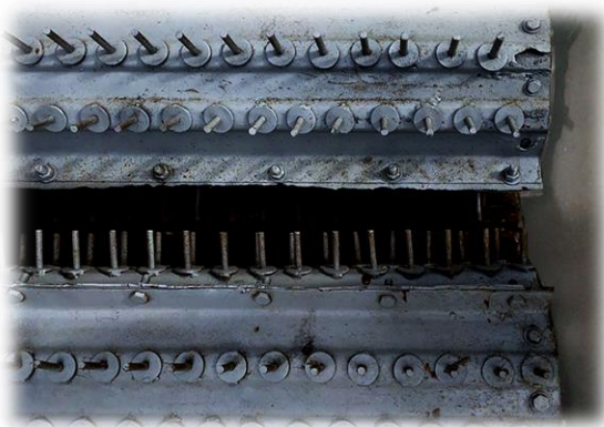
Figure 2. Appearances of peg drums with diameters of 8 mm (a), 10 mm (b) and 12 mm (c).
